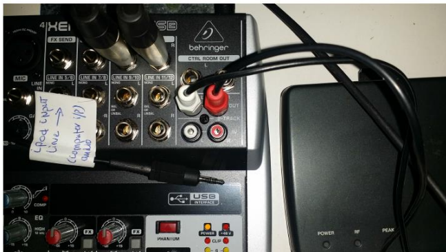
The red and white (RCA) plugs are used to play sound from a cellphone, laptop, CD player, etc.
